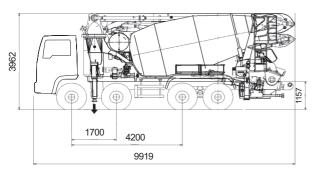
Dimensions varying according to truck assembly
